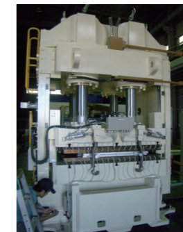
1,000 ton press for insulation sheet manufacture
